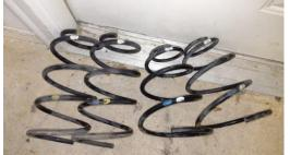
Porsche uses colored paint dots to denote various spring rates and shock rates. The blue/white and blue/yellow as well as the blue on the shocks indicate standard suspension. The sport springs have red dots. Quick way to tell if you already have sport suspension.
