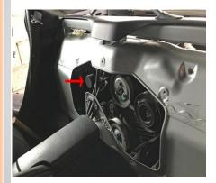
Red arrow shows where the alternator is on a 987.1 Cayman. The labor involved to remove and replace the alternator is always more expensive than a battery.
