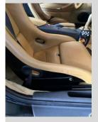
I assessed the required removal of the passenger seat and set about the task. As some of you know, I do not have the standard 996 seats but rather the optional GT3- style buckets. The seats nest in a frame which is then attached to the slider rails. Just four 3/8" bolts keep you from splattering the windshield when braking.
